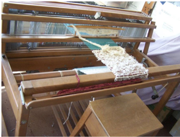
54" Walling loom, 46" weaving width. 4 harnesses, solid maple, custom-made by Bill Walling for Jan Hughes. 6 treadles and a bench. It's a sweet loom. Bench has damaged corner, but no rough edges. $800 obo Karen Dennis 561-4705
